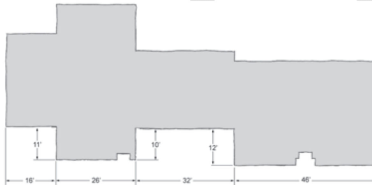
Example of building footprint massing and articulation that provides opportunities for functional open space and breaks in the visual scale of the building. Source: Contextual Design on Cape Cod | Design Guidelines for Large Scale Development
