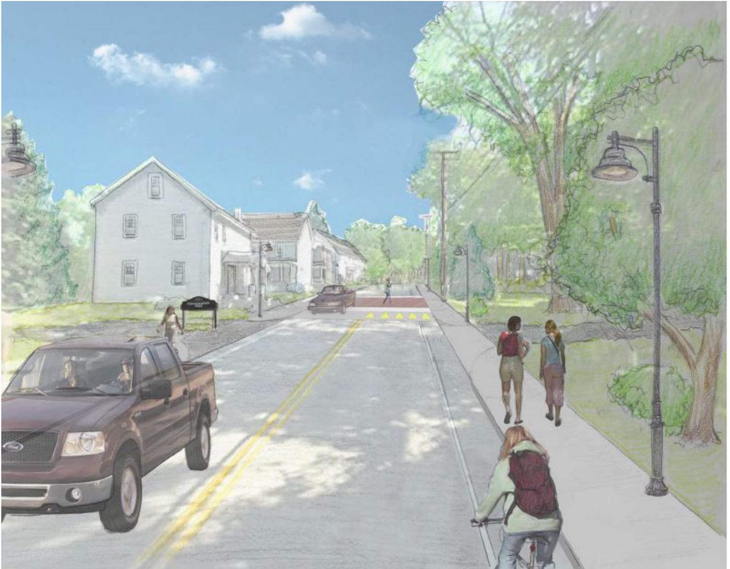
**Looking north on Gleasondale Road with sidewalks, period-appropriate lighting, raised crosswalks, and signage for the Gleasondale Mill. Note: Utility poles may be placed below-grade**
